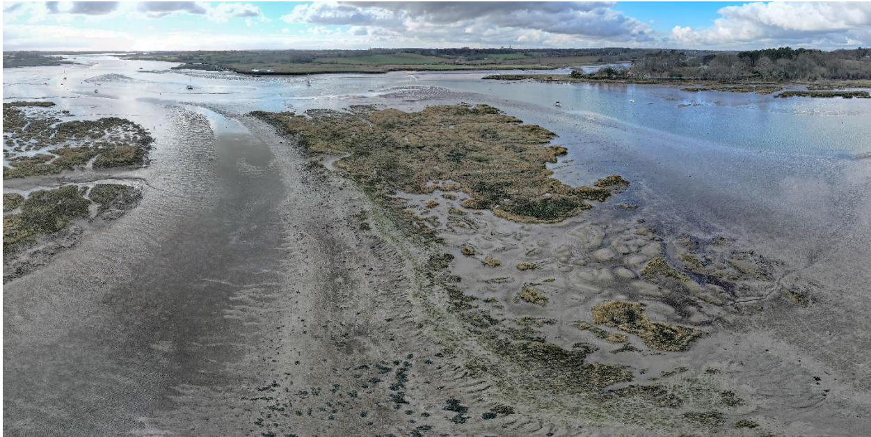
Recharge of sediment (deposited strip can be seen in the foreground) on Loder's Cut Island in the Deben Estuary – Jim Pullen.
